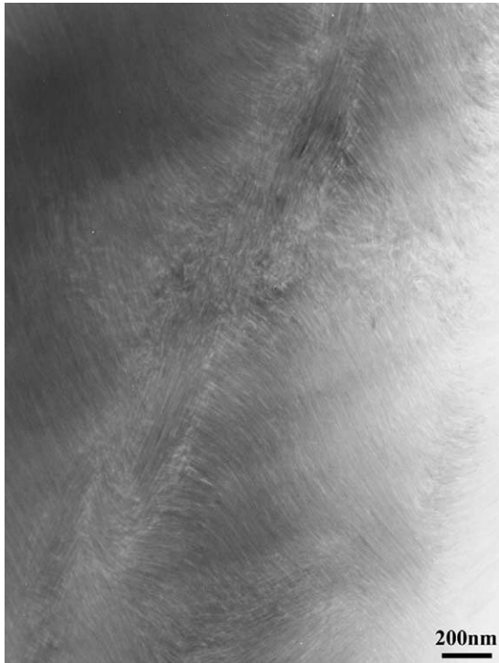
Fig. 14. TEM image of a fibrous zone composed of slightly curved and strongly oriented chrysotiles. A central narrow zone shows folded chrysotile fibres displaying a different and high-angle orientation.
